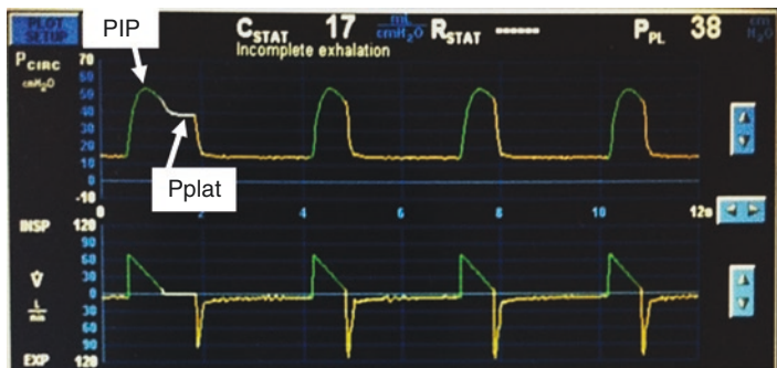
FIGURE 5.5 Ventilator screen showing the relationship between the peak inspiratory pressure (PIP) and the plateau pressure (Pplat.) The Pplat is only seen with an inspiratory hold maneuver
